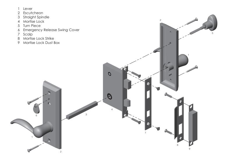
Note: Cut Shank on Turn Piece so that it goes halfway through the Mortise Lock. This will allow a space for the emergency release key to operate the Dead Bolt.
