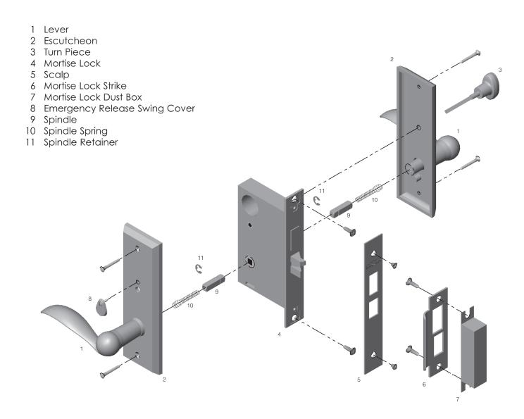
Note: Cut Shank on Turn Piece so that it goes halfway through the Mortise Lock. This will allow a space for the emergency release key to operate the Mortise Lock.
