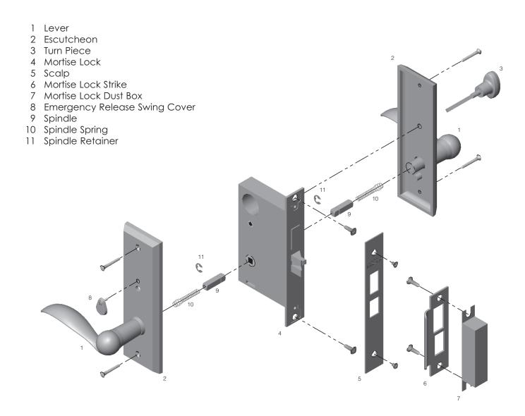
Note: Cut Shank on Turn Piece so that it goes halfway through the Mortise Lock. This will allow a space for the emergency release key to operate the Mortise Lock.
