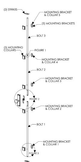
Step 1: attach bolt 2 & bolt 3 with machine screws provided. (see figure 1)
